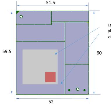
Label with FCC and IC ID information is placed on top of the module and is clearly visible.
