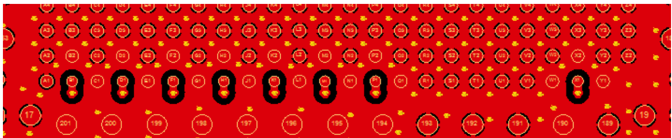
Figure 9-5: Antenna Pad Ground Cutout Recommended (Main Board, top layer/NAD side)
