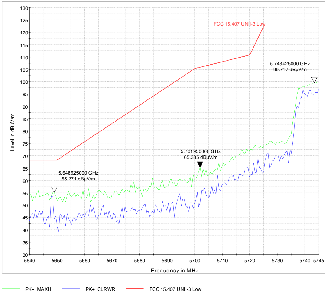
Figure 38: Low U-NII-3 band edge for 802.11n HT40+ MCS0 at Channel 151
