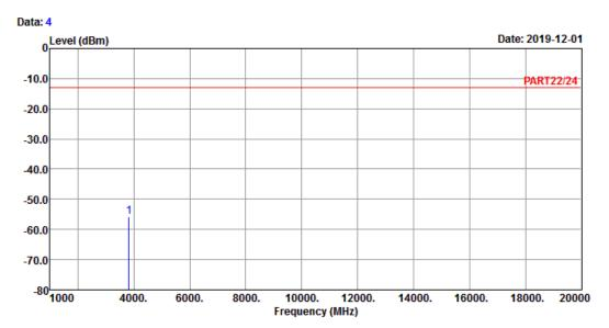
Site : 966 Chamber 5 Condition: PART22/24 VERTICAL Remark : WCDMA Band 2 Link\_H-CH
