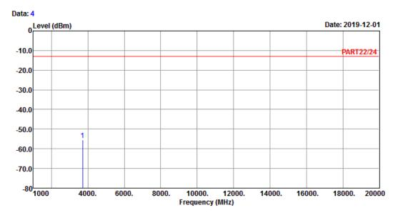
Site : 966 Chamber 5 Condition: PART22/24 VERTICAL Remark : WCDMA Band 2 Link\_L-CH
