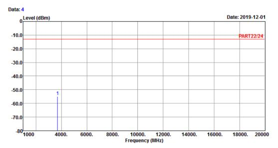
Site : 966 Chamber 5 Condition: PART22/24 VERTICAL Remark : PCS 1900 Link\_L-CH
