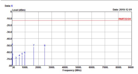
Site : 966 Chamber 5 Condition: PART22/24 VERTICAL Remak : GSM 850 Link\_L-CH
