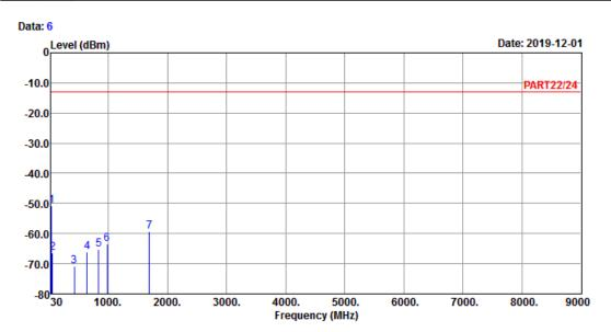
Site : 966 Chamber 5 Condition: PART22/24 VERTICAL Remark : WCDMA Band V Link\_H-CH
