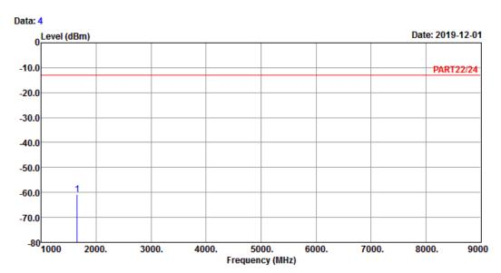
Site : 966 Chamber 5 Condition: PART22/24 VERTICAL Remark : WCDMA Band V Link\_L-CH
