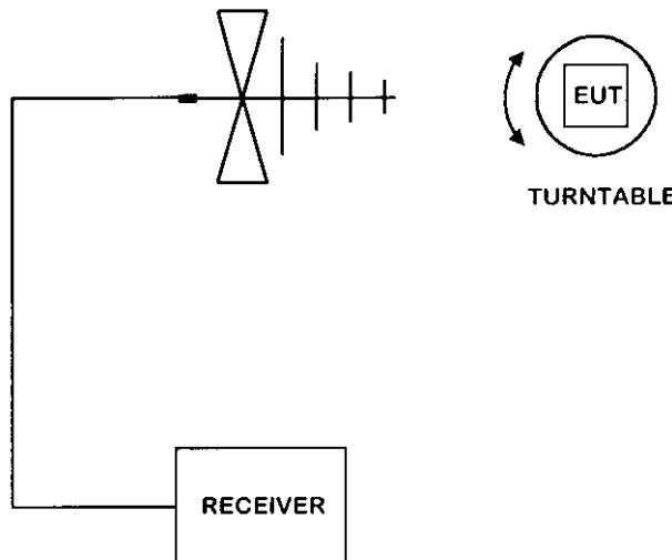
TEST SETUP FOR RADIATED EMISSIONS TEST
