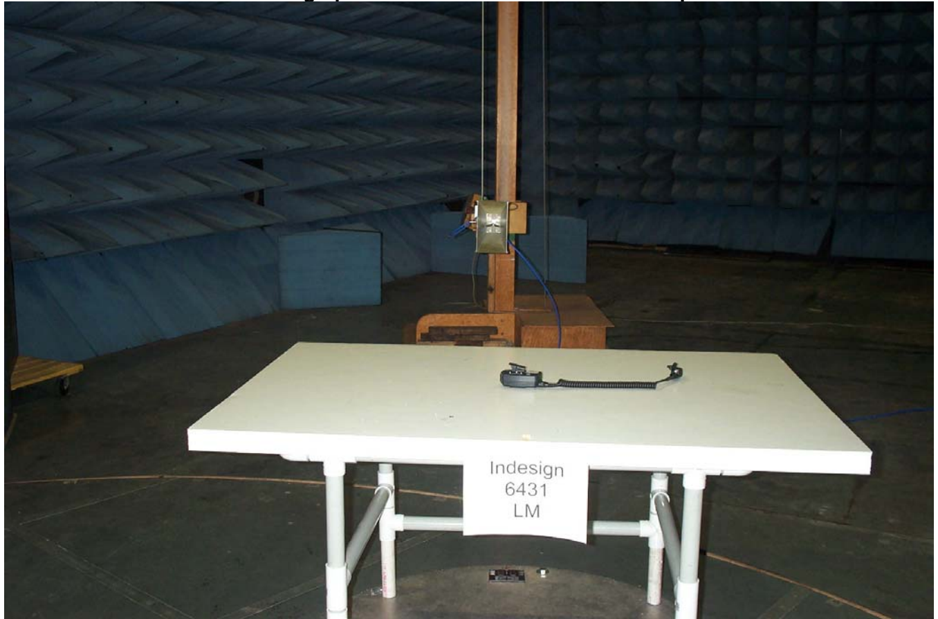
Photograph of Radiated Emissions Test Setup
