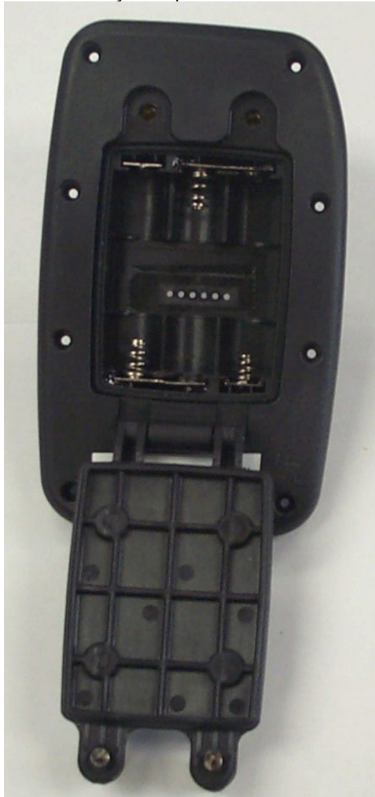
Battery Compartment of EUT
