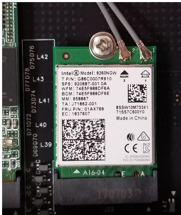
Figure 5 NIM Vital Console, Model NIM4CM01, Internal View, Intel Module 9260NGW
