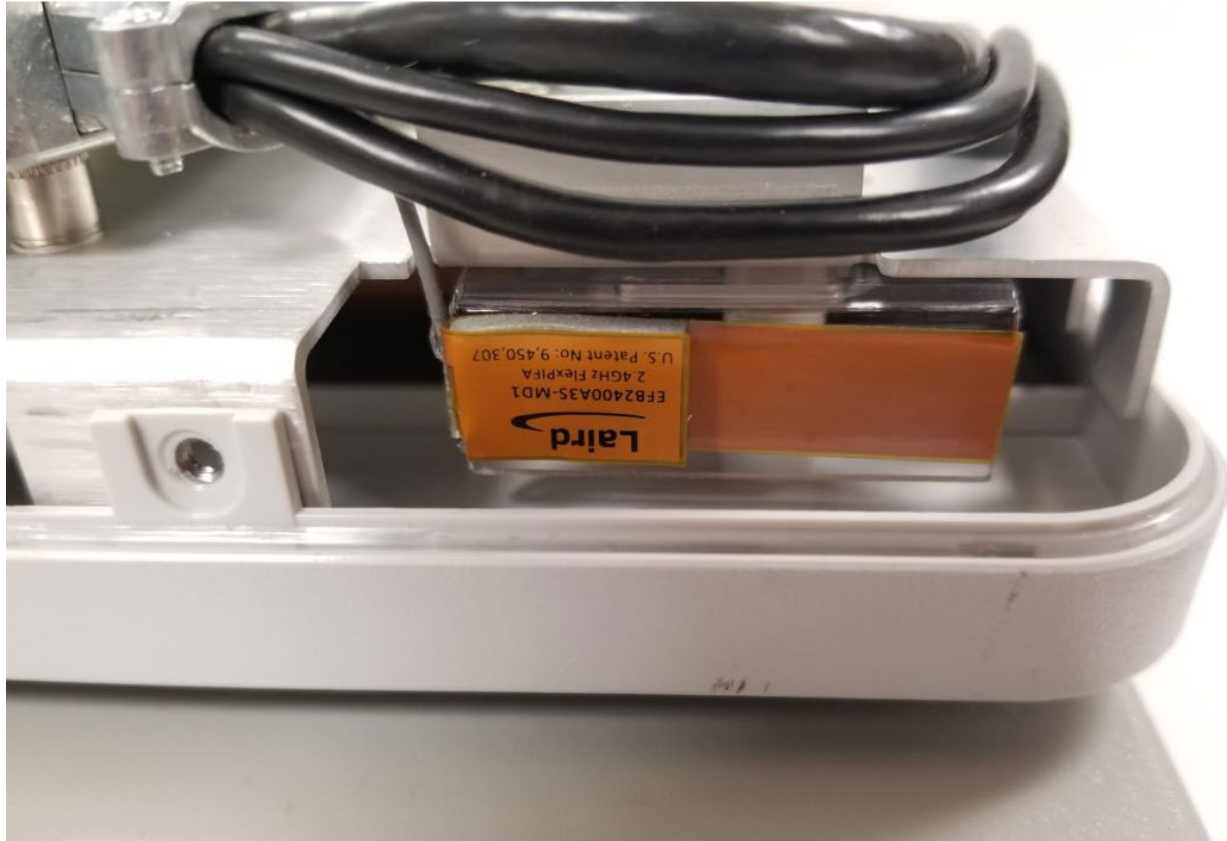
Figure 9 NIM Vital Console, Model NIM4CM01, Internal View, Lower Right Antenna
