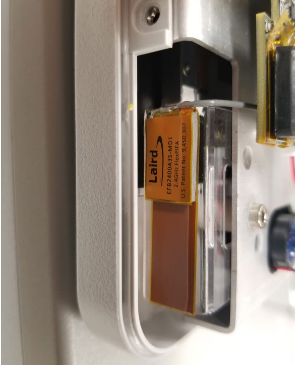
Figure 8 NIM Vital Console, Model NIM4CM01, Internal View, Lower Left Antenna
