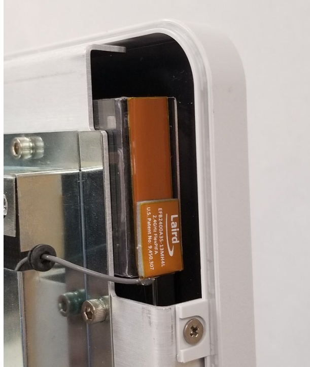
Figure 7 NIM Vital Console, Model NIM4CM01, Internal View, Upper Right Antenna
