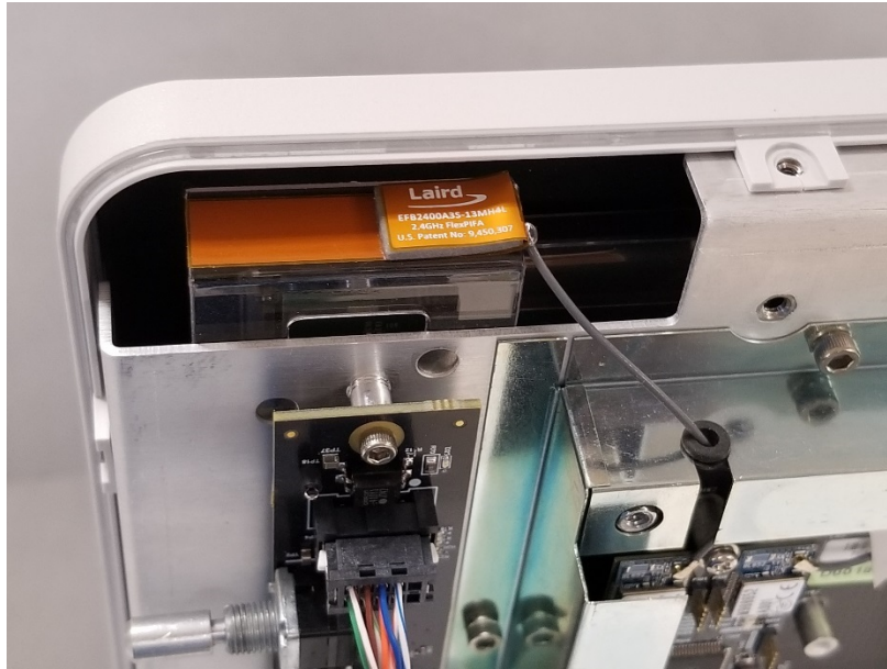
Figure 6 NIM Vital Console, Model NIM4CM01, Internal View, Upper Left Antenna
