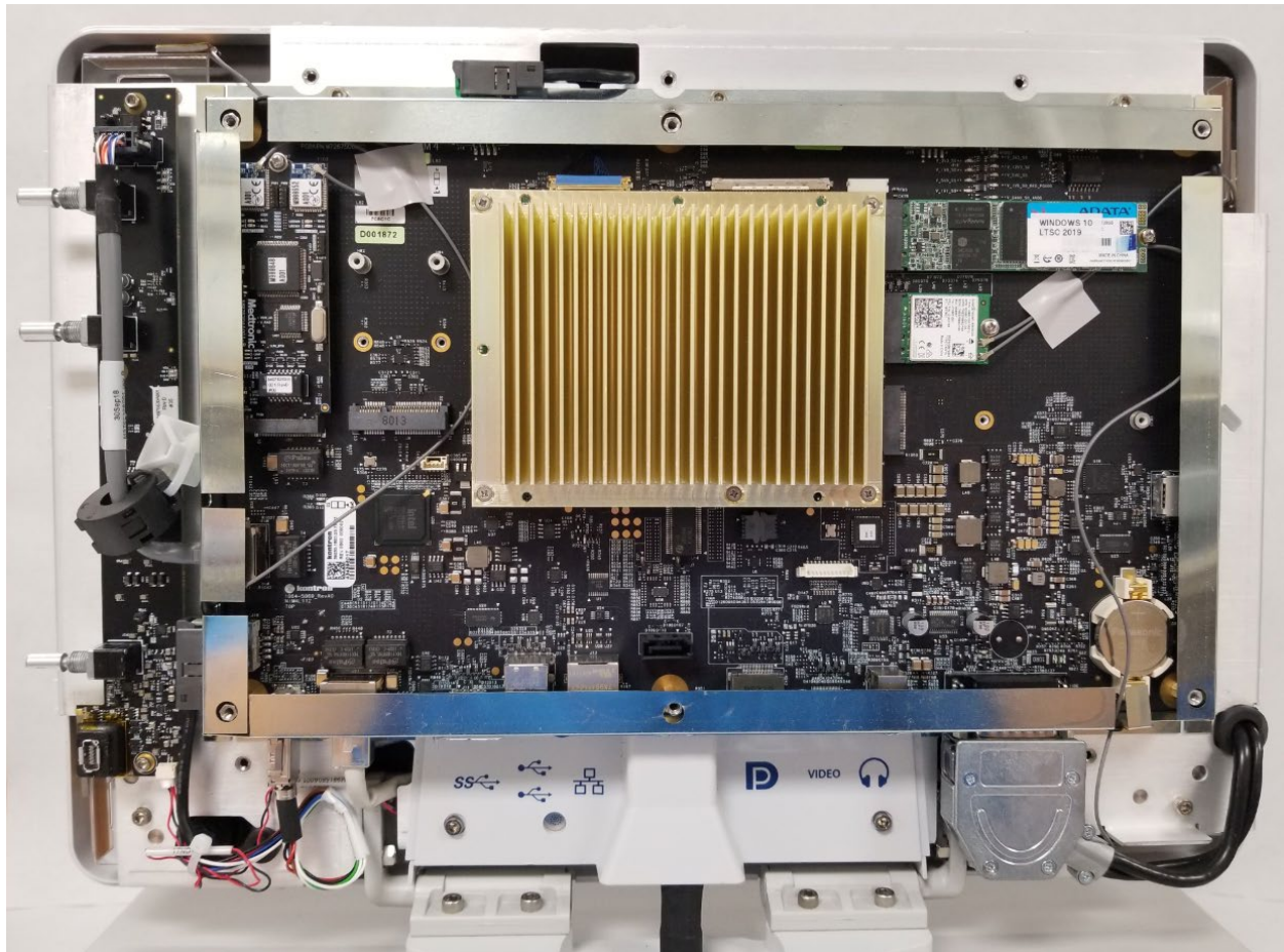
Figure 2 NIM Vital Console, Model NIM4CM01, Internal View, Main Board
