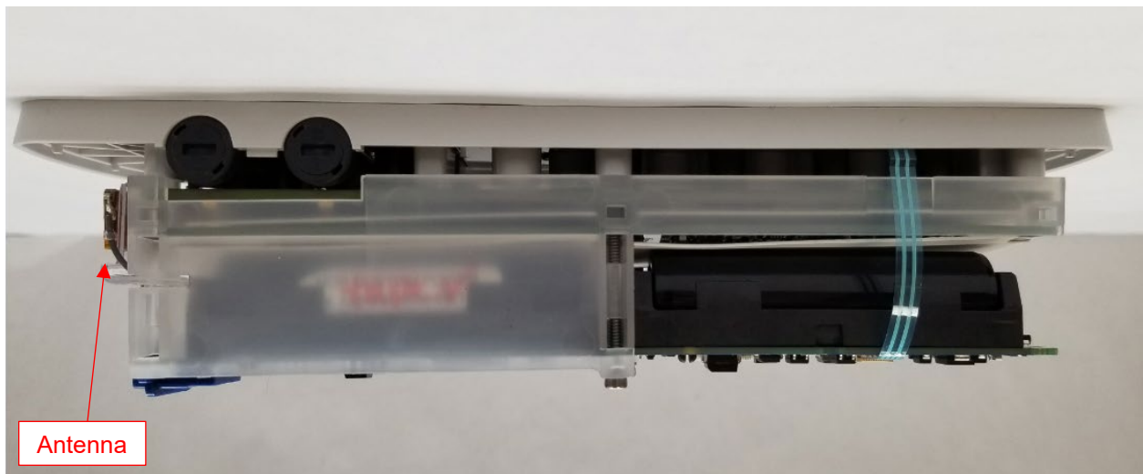
Figure 6 NIM Vital Patient Interface NIM4CPB1 Right Side View with Bottom Enclosure off
