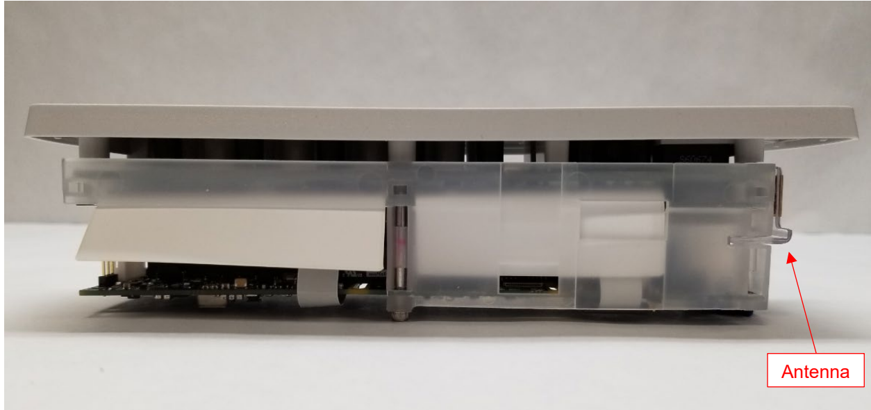
Figure 5 NIM Vital Patient Interface NIM4CPB1 Left Side View with Bottom Enclosure off
