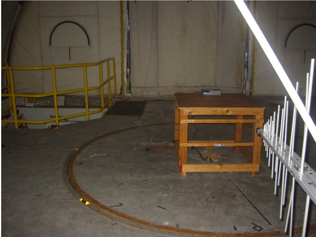
Radiated Emissions Setup Photo 2
