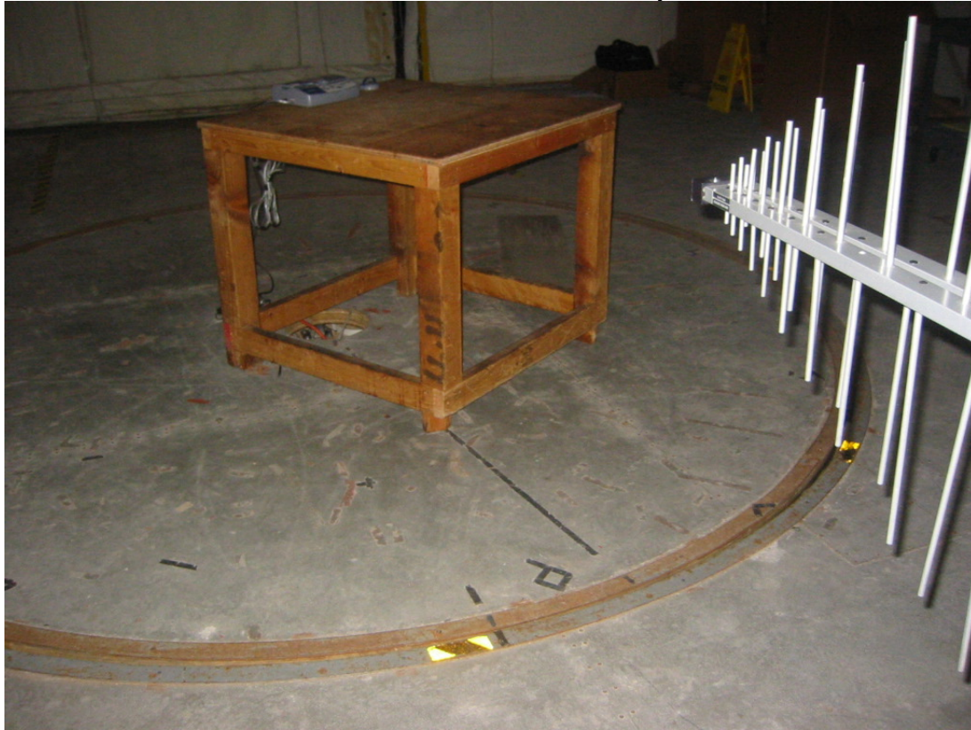
Radiated Emissions Setup Photo 3
