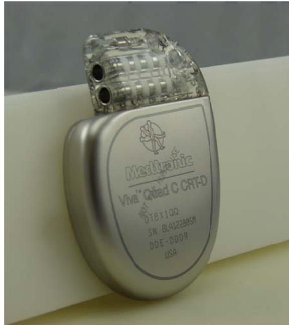
Figure 1: Medtronic Viva Implantable Cardiac Rhythm Disease Management Device
