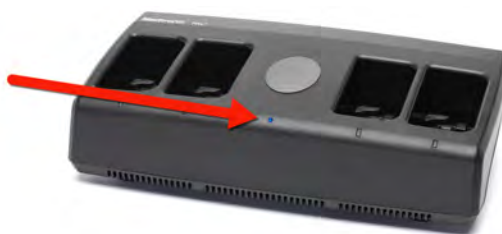
Figure 82: Battery Charger blue status Indicator Light
