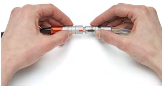
Figure 48: Push the driveline connector into the port
