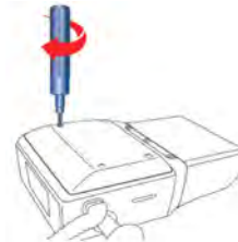
Figure 206: Tighten back cover
