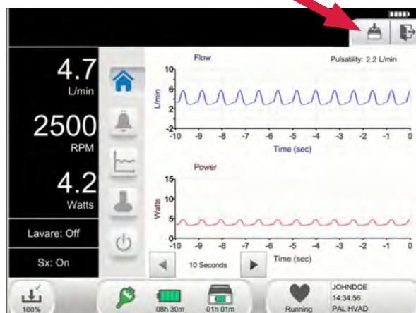
Figure 172: Screen indicating the controller is ready for software upgrade
