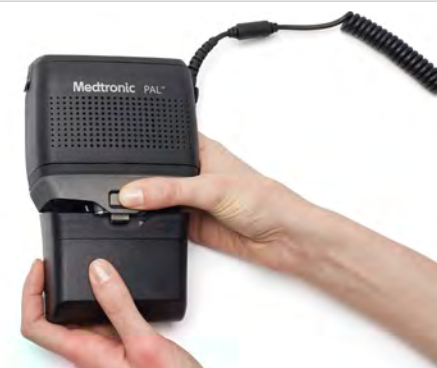
Figure 70: Press the “Battery Release” button
