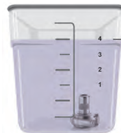
Figure 178: Submerged HVAD Pump
