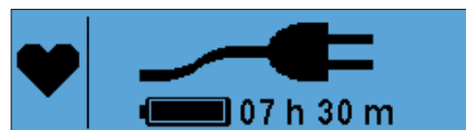
Figure 18: Example of navigation button (heart symbol) and display of controller system information
