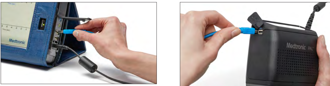
Figure 164: Data cable from monitor to controller
