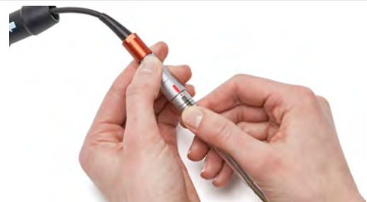
Figure 109: Pinch the grooved area of the controller Coiled Cable connector
