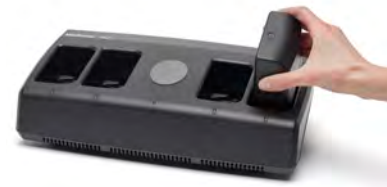
Figure 79: Place battery into charging bay
