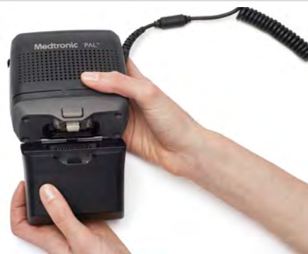
Figure 71: Detach the battery tabs
