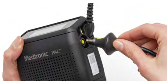
Figure 60: Align the cable connector with the controller power connector port
