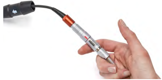
Figure 107: Grasp the pump driveline cable
