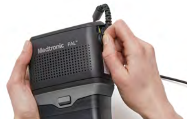
Figure 64: Cover the port with dust cover
