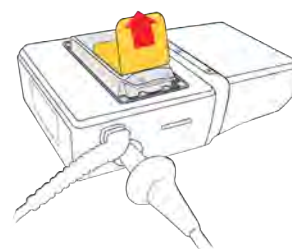
Figure 201: Disconnect internal battery
