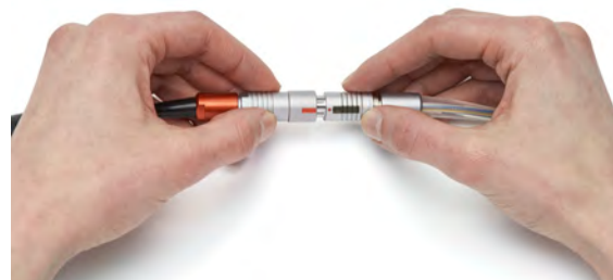
Figure 112: Push the driveline connector into the port
