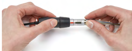
Figure 113: Slide the cover over connectors
