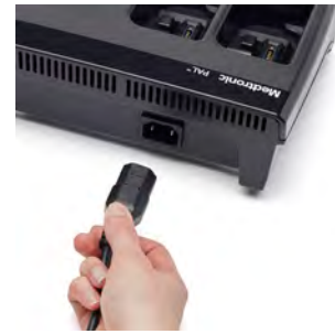
Figure 76: Connect the AC power cord
