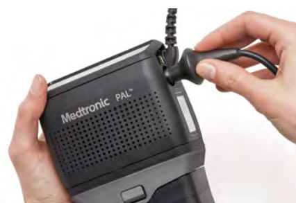
Figure 63: Pull the power cord out
