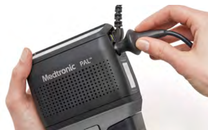
Figure 75: Push cable into controller
