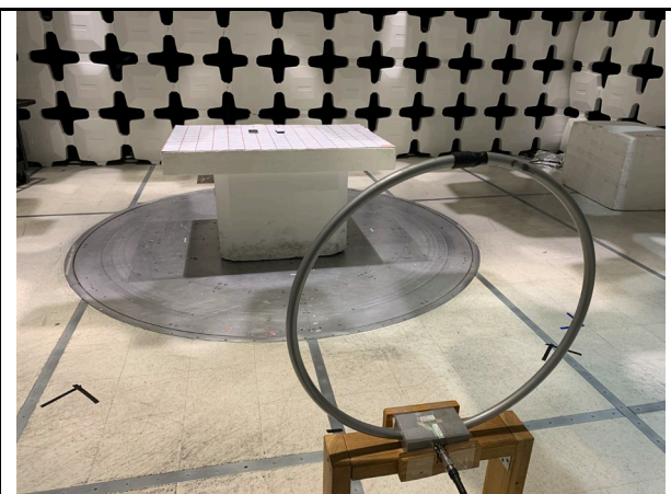
Radiated Emission Test below 30MHz Rear View
