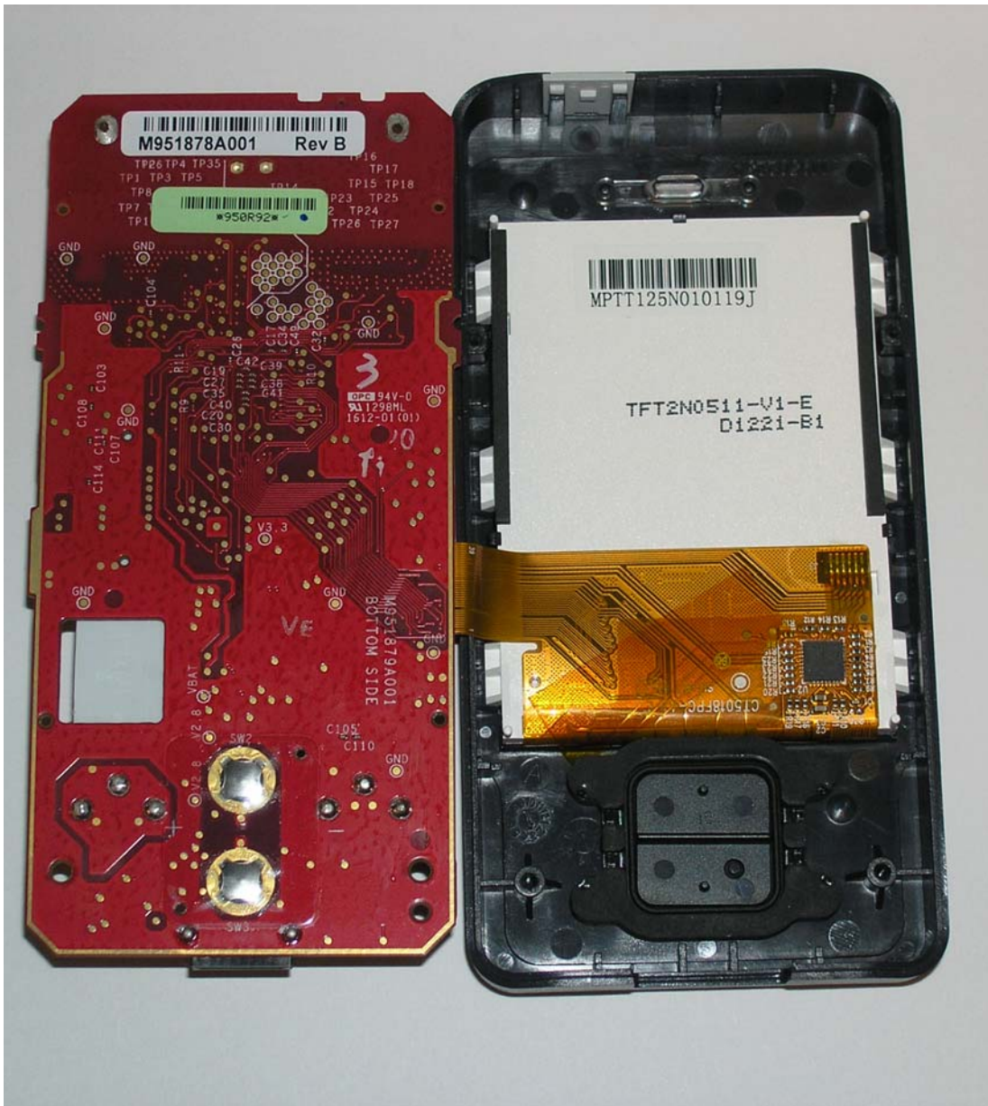
PTM Intellis Model 97745 Internal View of LCD with Flex Circuit
