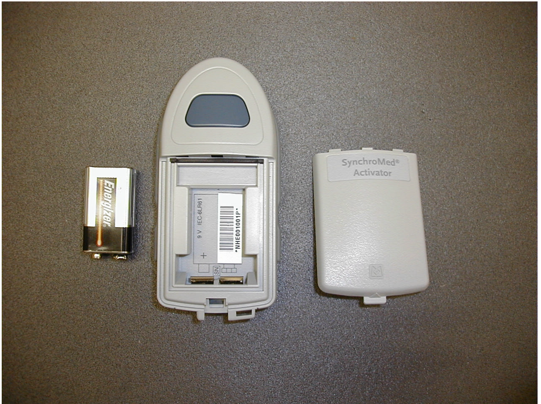
Disassembly – Front cover off, battery out
