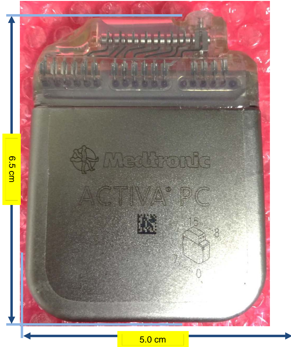
Figure 1: ACTIVA® PC, Model: 37601, Front View (with dimensions)
