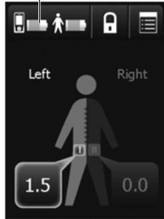
Figure 78. Viewing the battery status on the Home screen.
