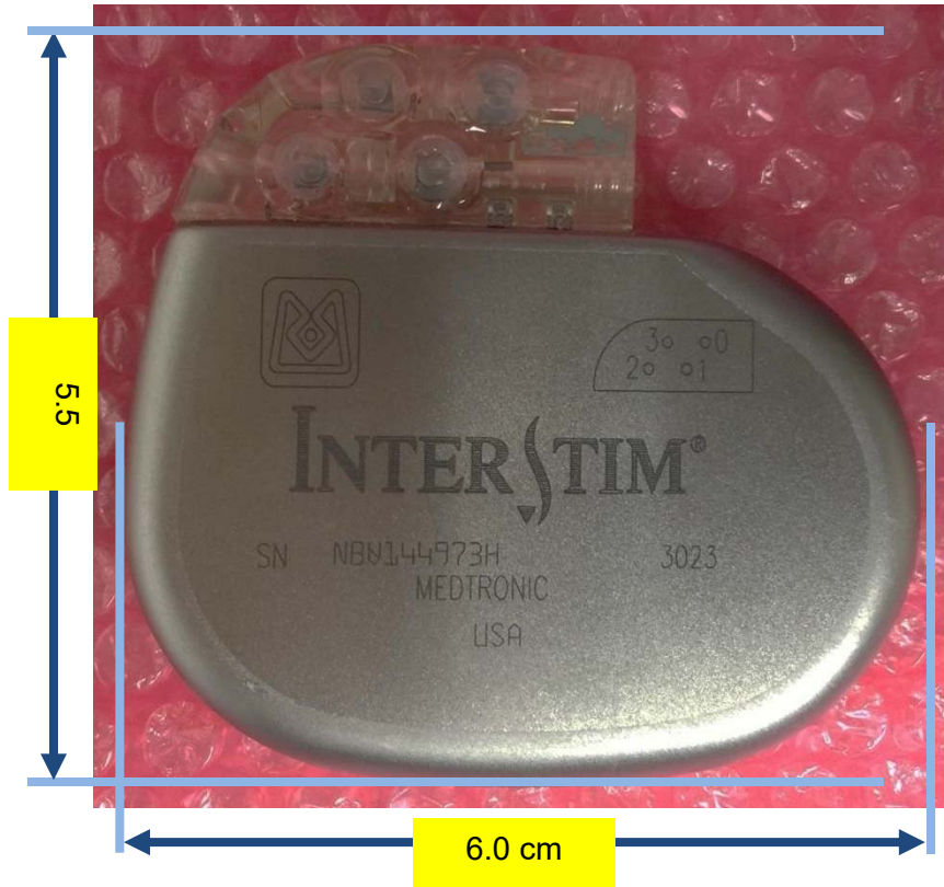
Figure 1: InterStim® , Model: 3023, Front View (with dimensions)
