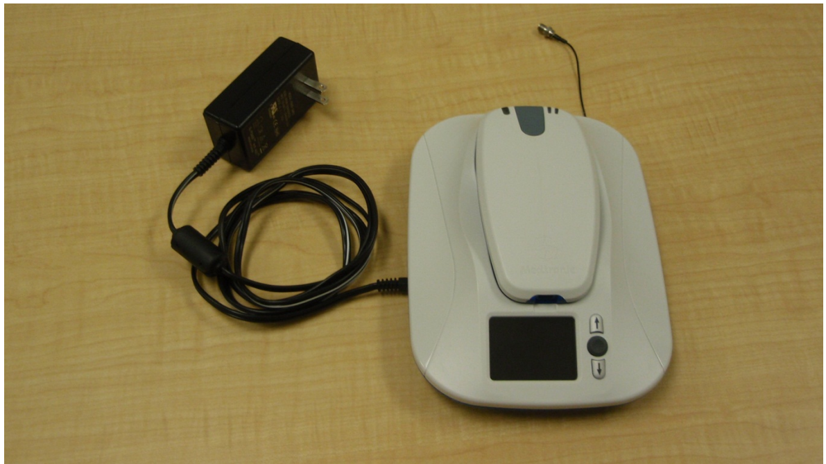
FIGURE 3: VISUAL OF EUT WITH RF CABLE AND CONNECTOR
