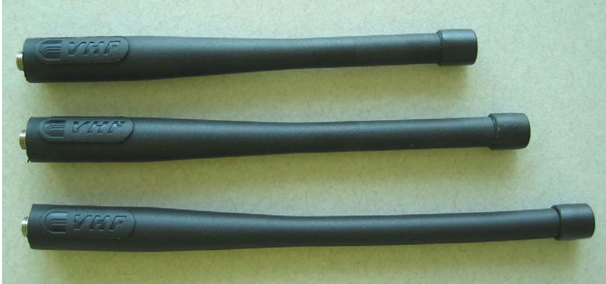
Figure 8: U3 Dual band (GPS/VHF) Antennas (High, Mid, Low Band)
