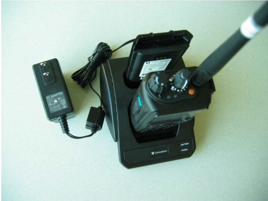
Figure 3: Battery Charger with U3 and battery
