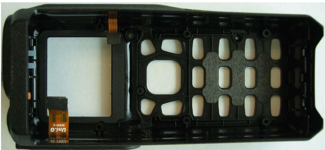
Figure 19: Plastic housing with Accessory FPC and PTT FPC
