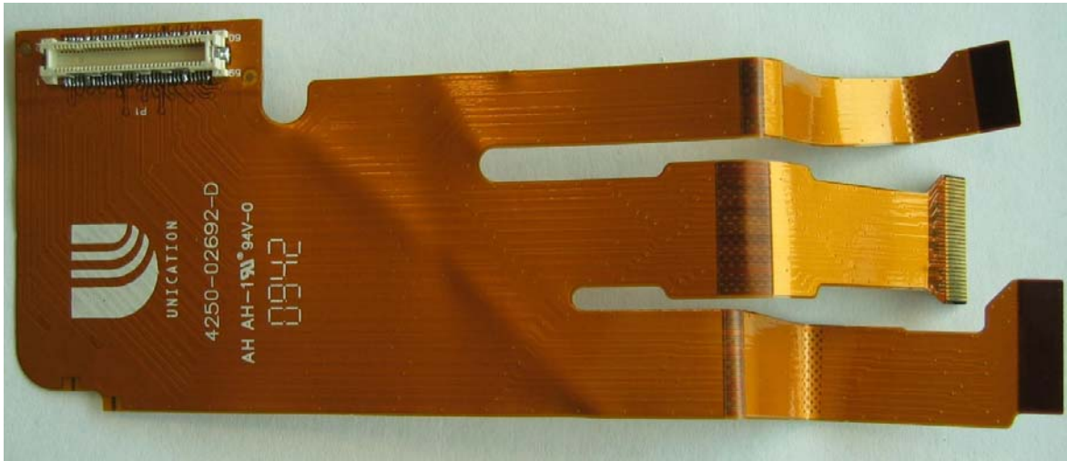
Figure 17: Keyboard interconnect FPC bottom
