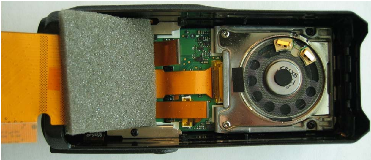
Figure 2 U3 Internals with main PCB removed - right side
