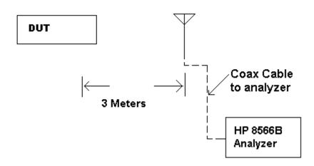
METHOD OF MEASUREMENT: The procedure used was ANSI standard C63.4-2003 & the FCC/OET Guidance on Measurements for Spread Spectrum Systems – Public Notice DA 00-705 dated March  $30^{th}$ , 2000.
