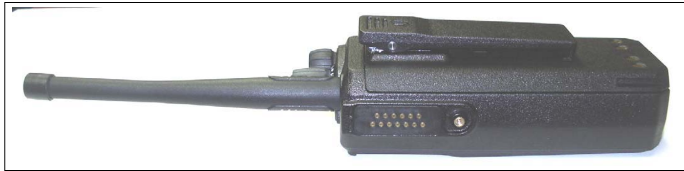
Side view of DUT with Belt-Clip Accessory & Detachable Whip Antenna
