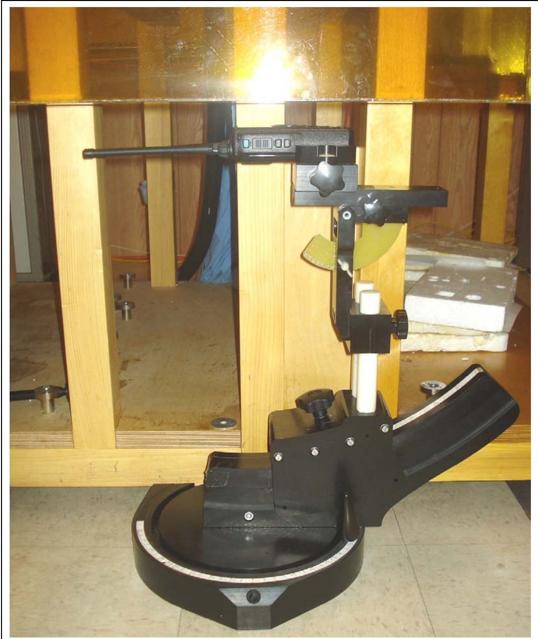
Face-held Configuration - DUT with 2.5 cm spacing from front keypad side of radio to planar phantom
