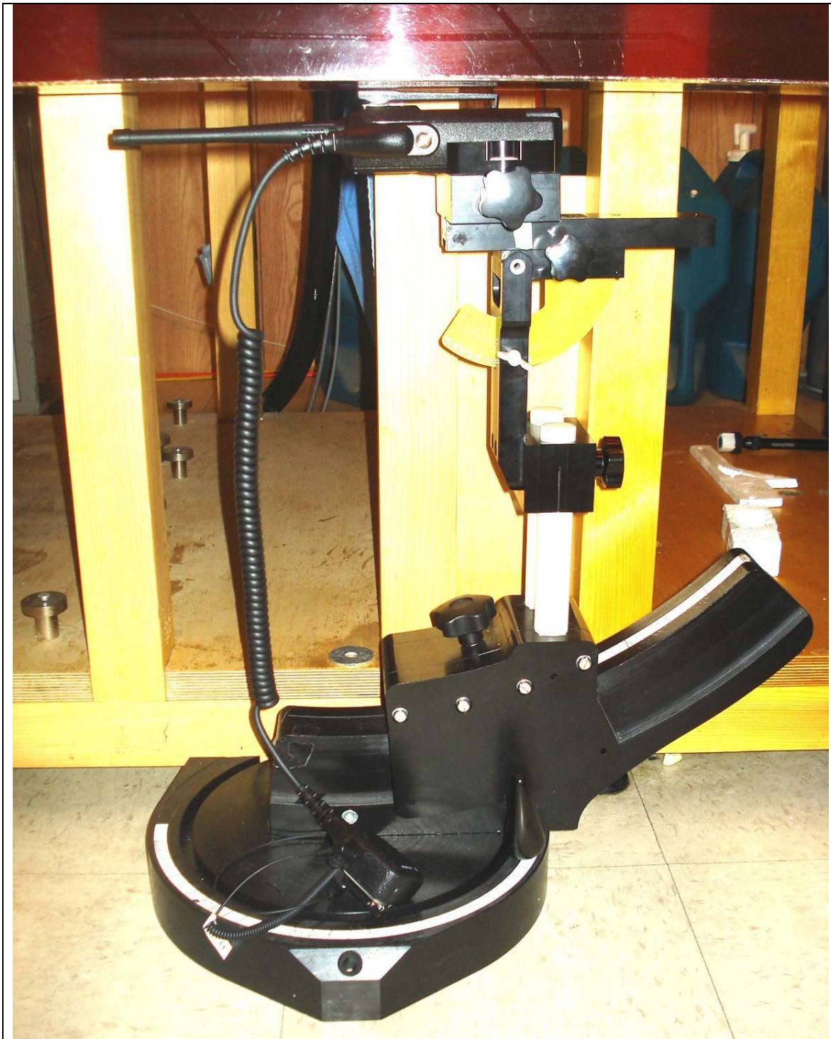
Body-worn Configuration - DUT with Belt-Clip Accessory & Speaker-Microphone with Earpiece Audio Accessory
