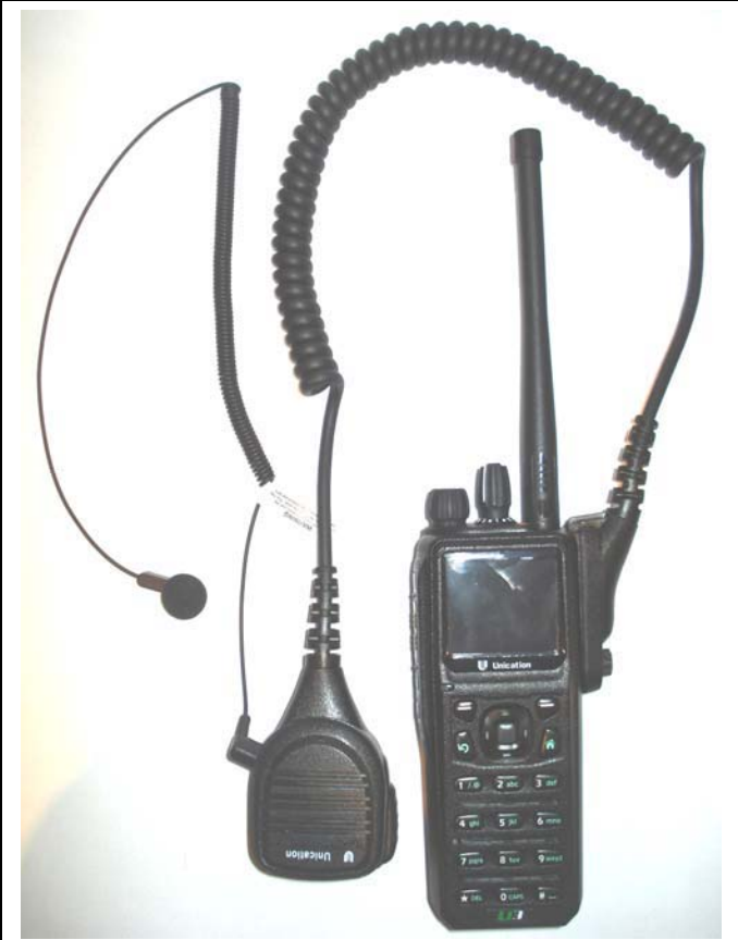
Front of DUT with Speaker-Microphone (P/N: 7106-00009-02) and Earpiece (P/N: 7106-00010) audio accessories
