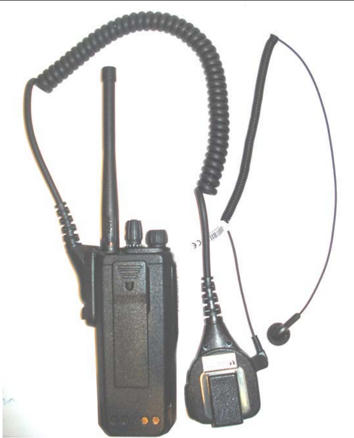
Back of DUT with Speaker-Microphone (P/N: 7106-00009-02) and Earpiece (P/N: 7106-00010) audio accessories
