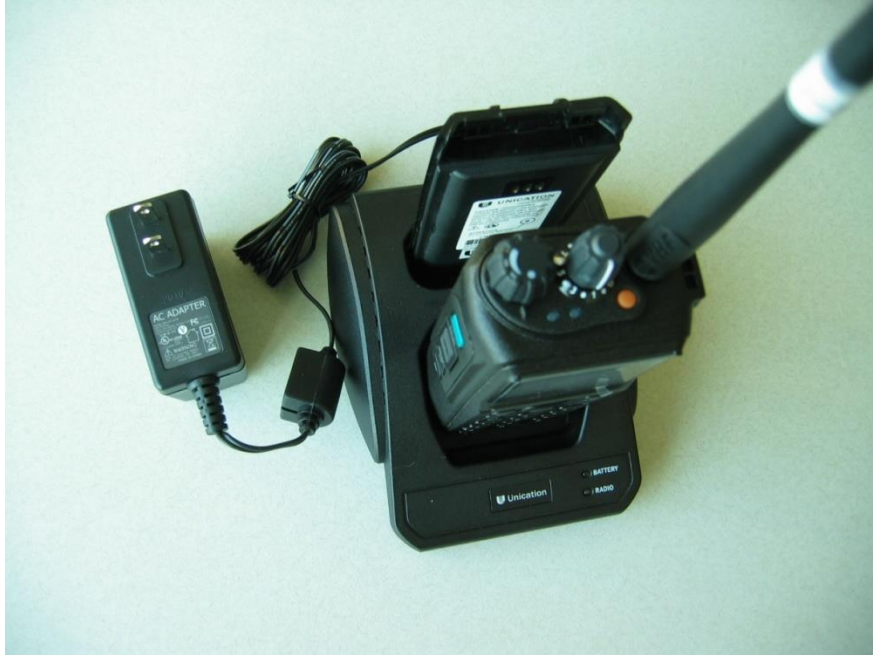
Figure 3: Battery Charger with U3 and battery
