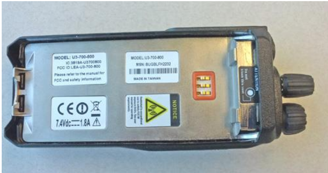
Figure 6: U3 back with battery removed
