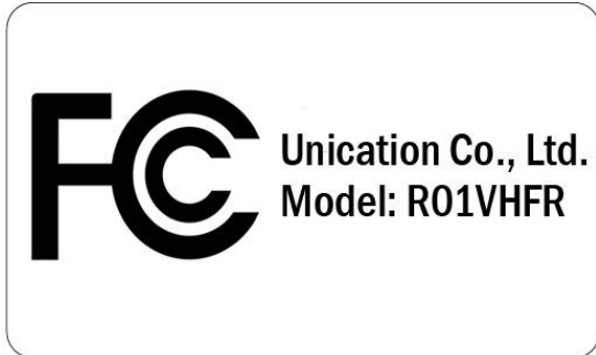
Figure 3: FCC Declaration of Conformity (DoC) Identification Label (Part 15)
