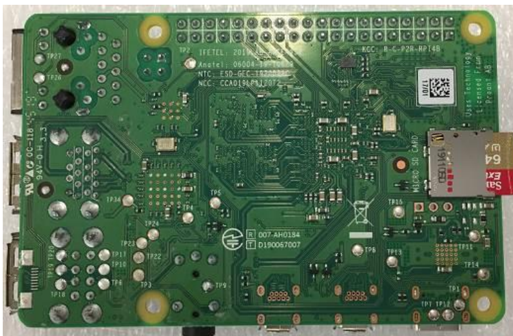
Figure 64: Raspberry PI 4 Model B PCBA Bottom View
