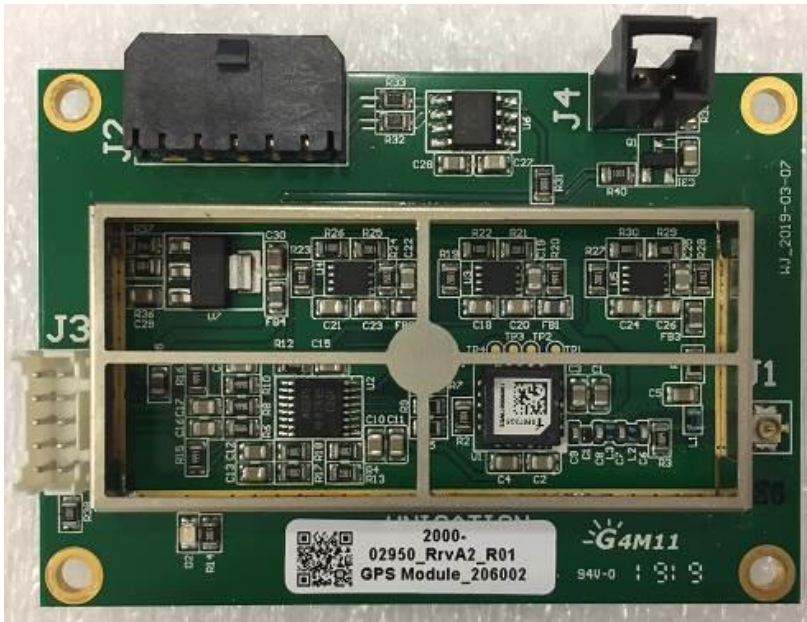
Figure 60: GPS PCBA Top View (Shield Cover Removed)
