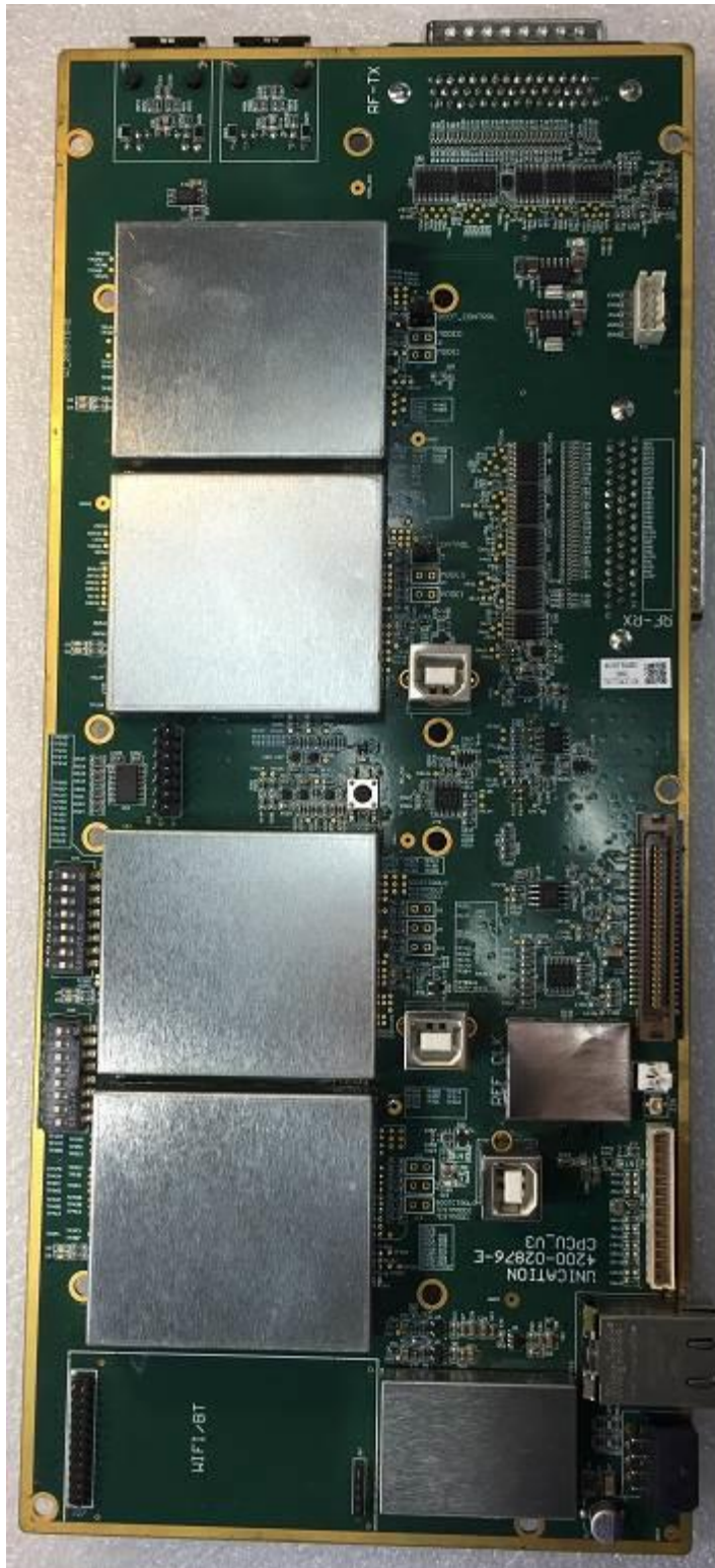
Figure 6: RX CPCU PCB Top View with shield covers installed
