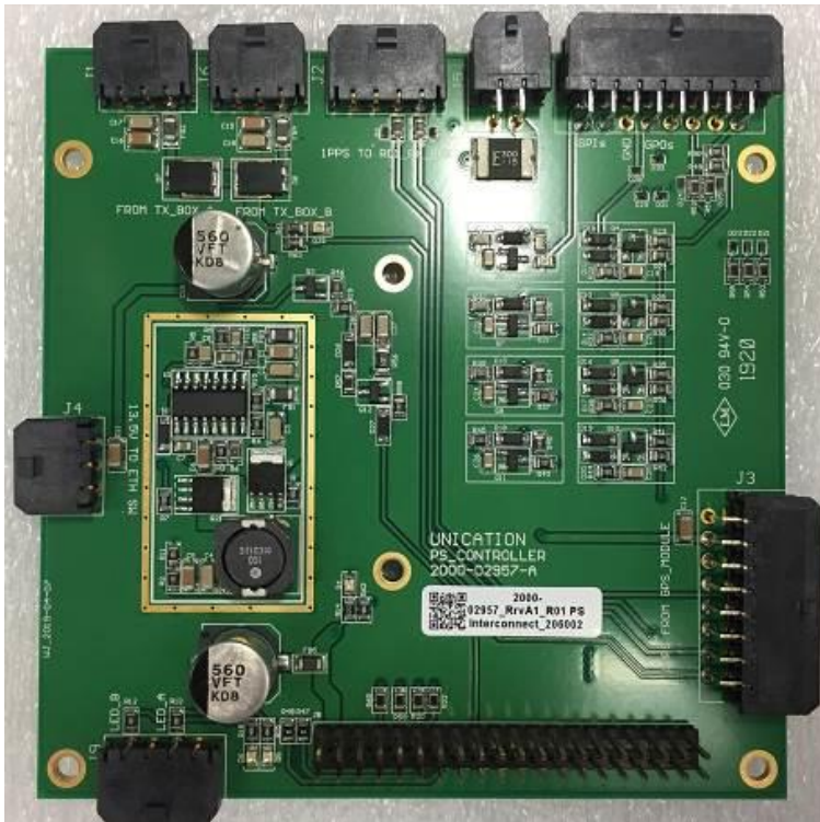
Figure 58: PS Controller PCBA Top View
