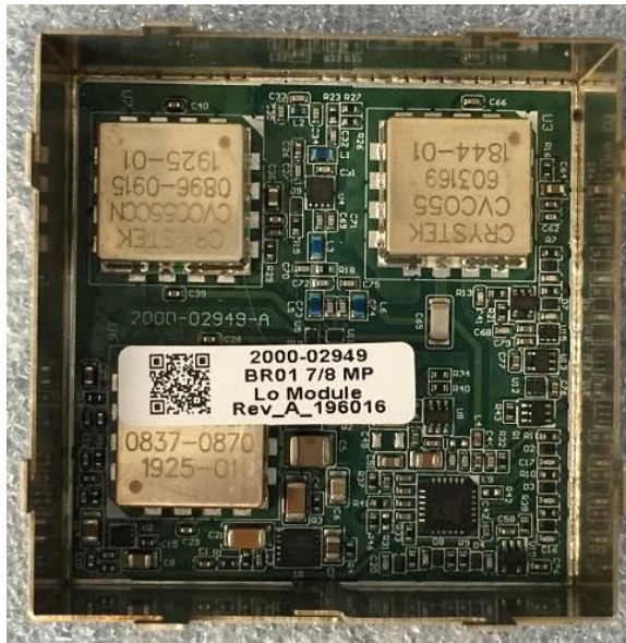
Figure 17: 700/800MHz Local Oscillator PCB Top View (shield cover removed)
