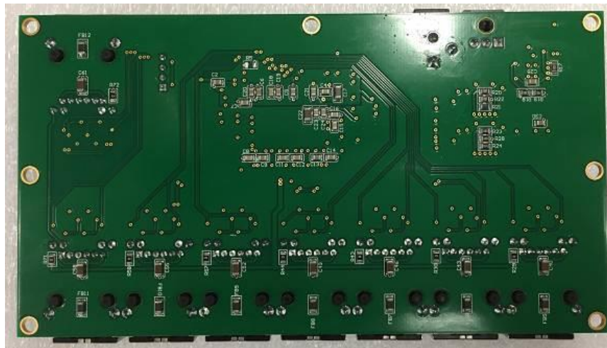
Figure 57: Ethernet Switch PCBA Bottom View
