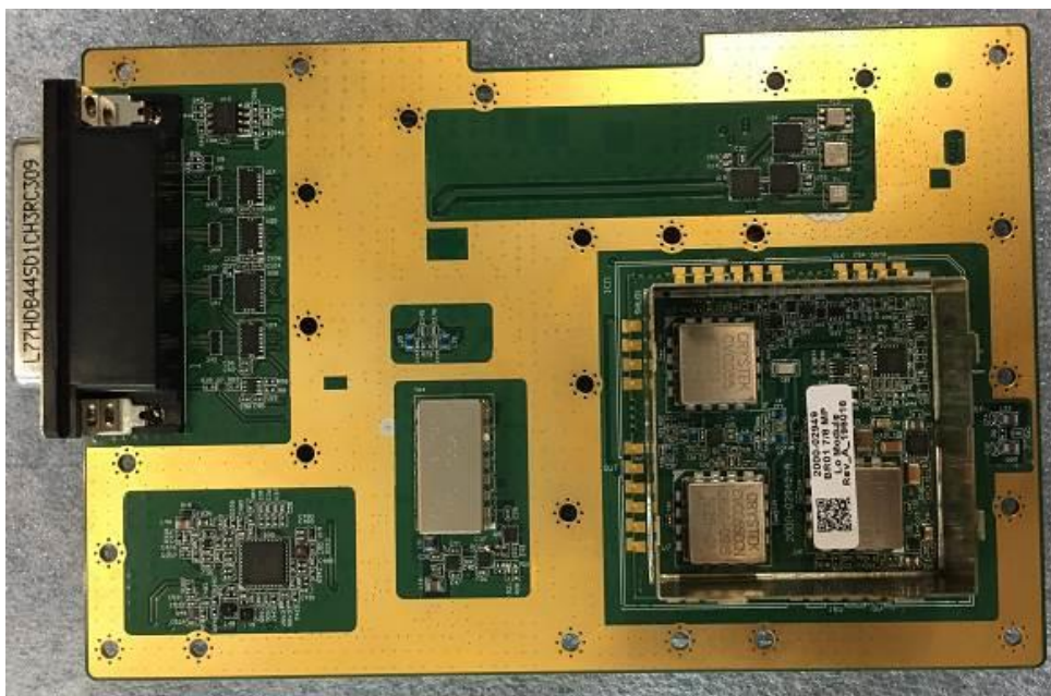
Figure 16: RX 700/800MHz Receiver PCB Bottom View (shield cover removed)
