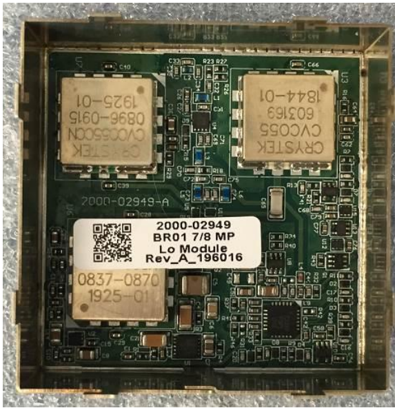
Figure 47: 700/800MHz Local Oscillator PCB Top View (shield cover removed)
