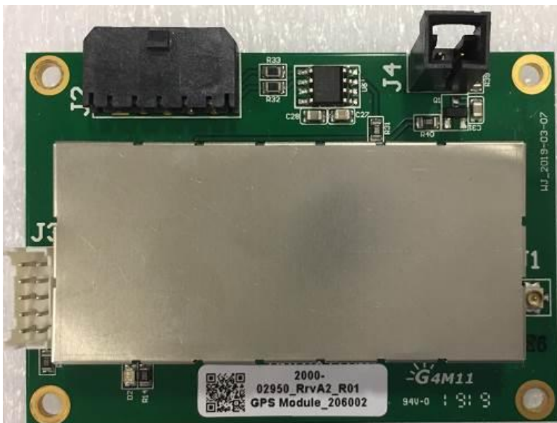
Figure 61: GPS PCBA Top View Shield Cover Installed
