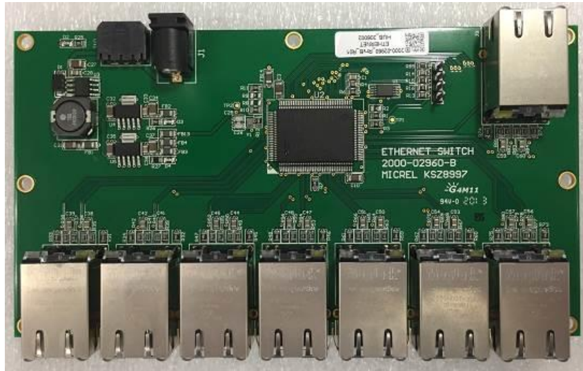
Figure 56: Ethernet Switch PCBA Top View
