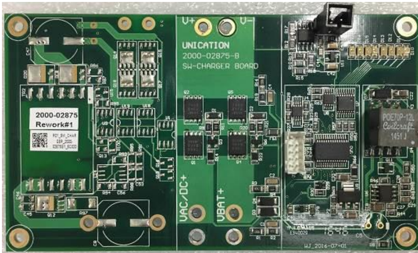
Figure 31: PS Switcher PCBA Top View
