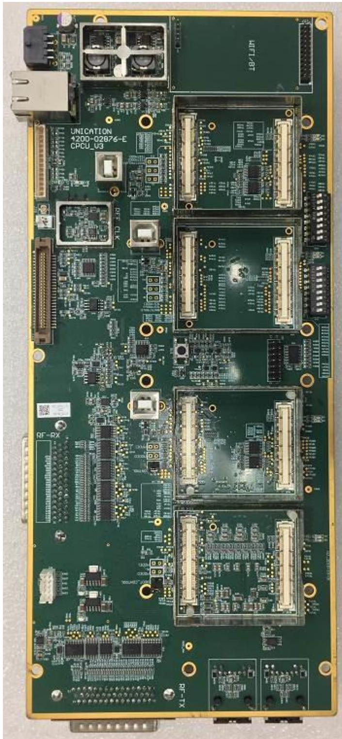
Figure 4: RX CPCU PCB Top View (shield covers removed)
