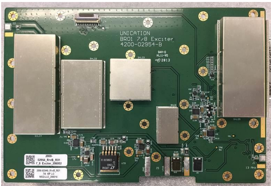
Figure 46: TX 700/800MHz Exciter PCB with Shields
