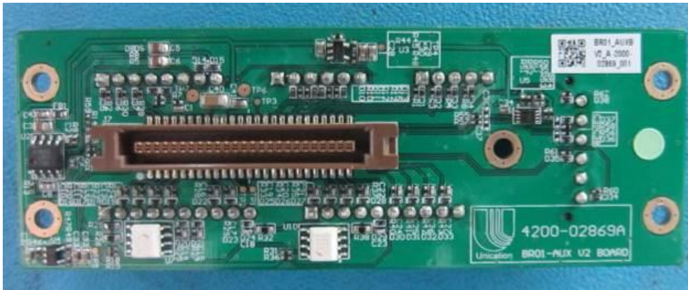
Figure 13: RX AUX V2 PCB Top View
