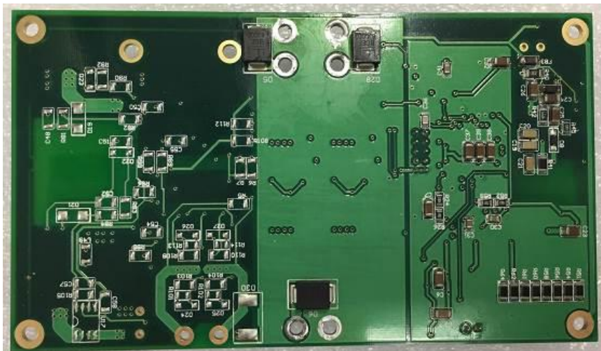
Figure 32: PS Switcher PCBA Bottom View
