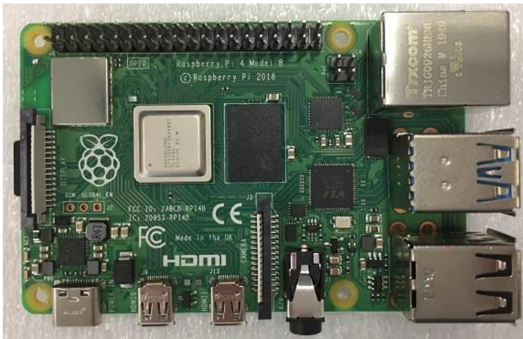
Figure 63: Raspberry PI 4 Model B PCBA Top View
