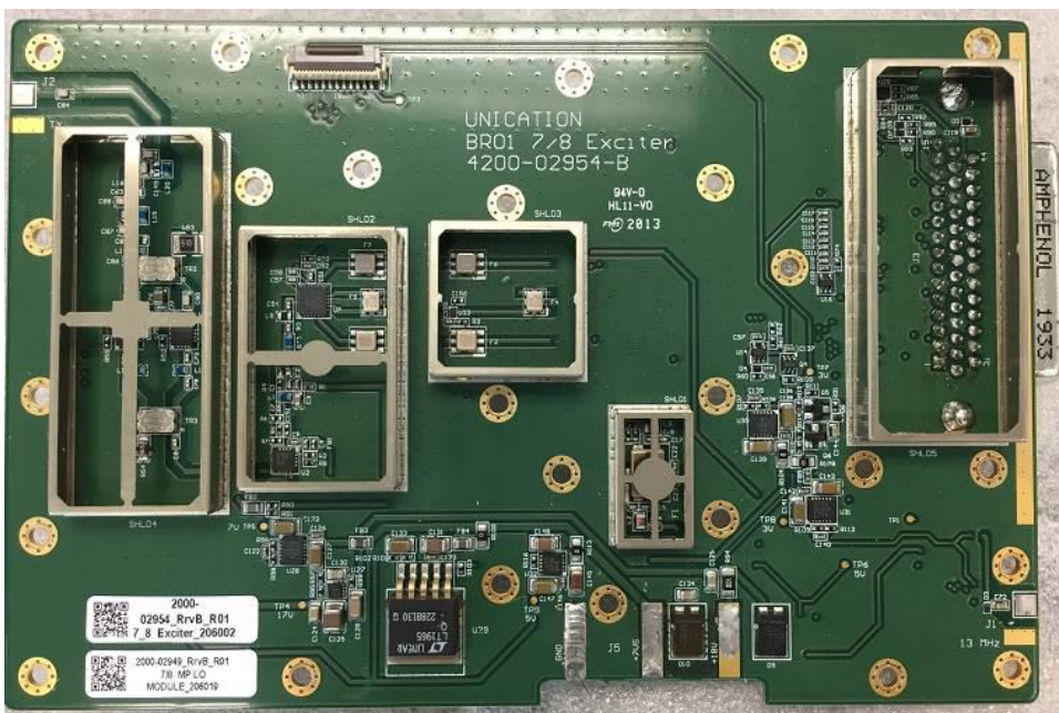
Figure 44: TX 700/800MHz Exciter PCB Top View
