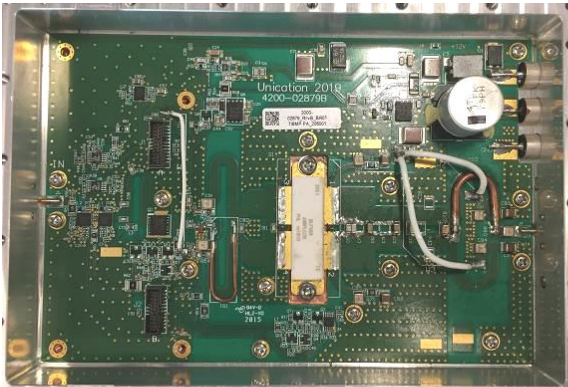
Figure 38: TX 700/800MHz PA PCBA Top View
