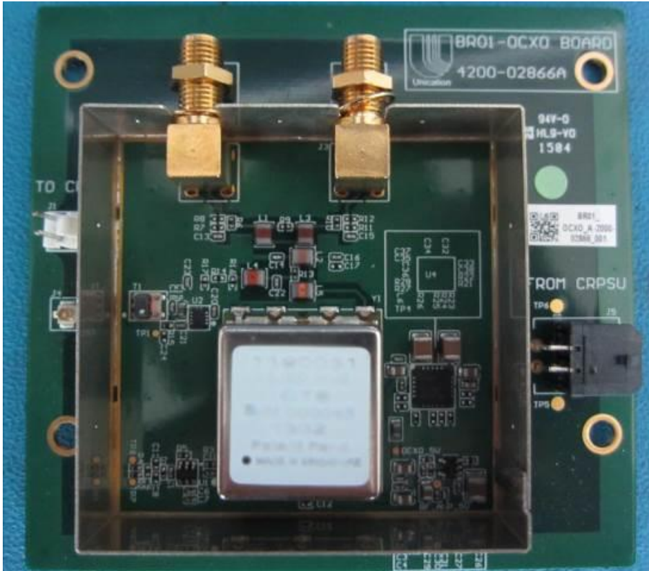
Figure 8: RX OCXO PCB Top View (shield cover removed)
