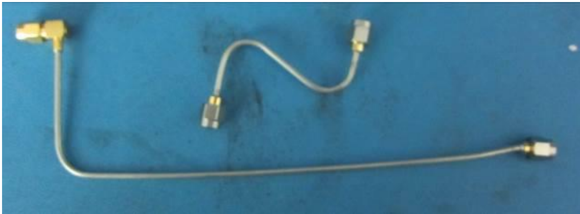
Figure 22: RX RF Coax Assemblies
