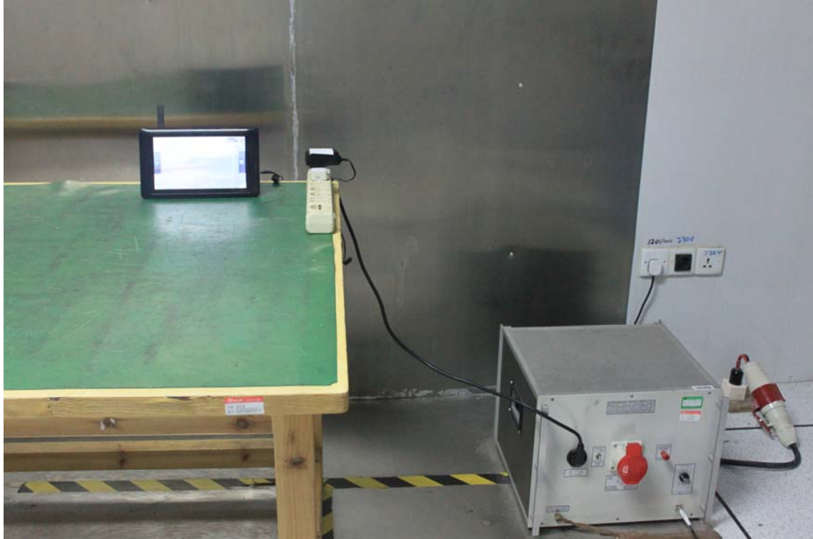
Photograph – Conducted Emission Test Setup
