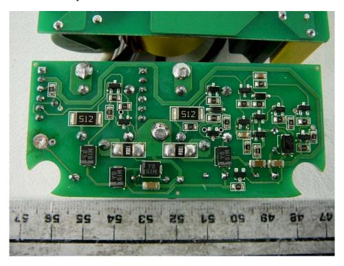
15.10 EUT – Power Supply PCB Assembly Front View
