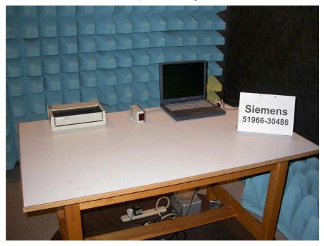
EUT in horizontal position- bottom side on table
