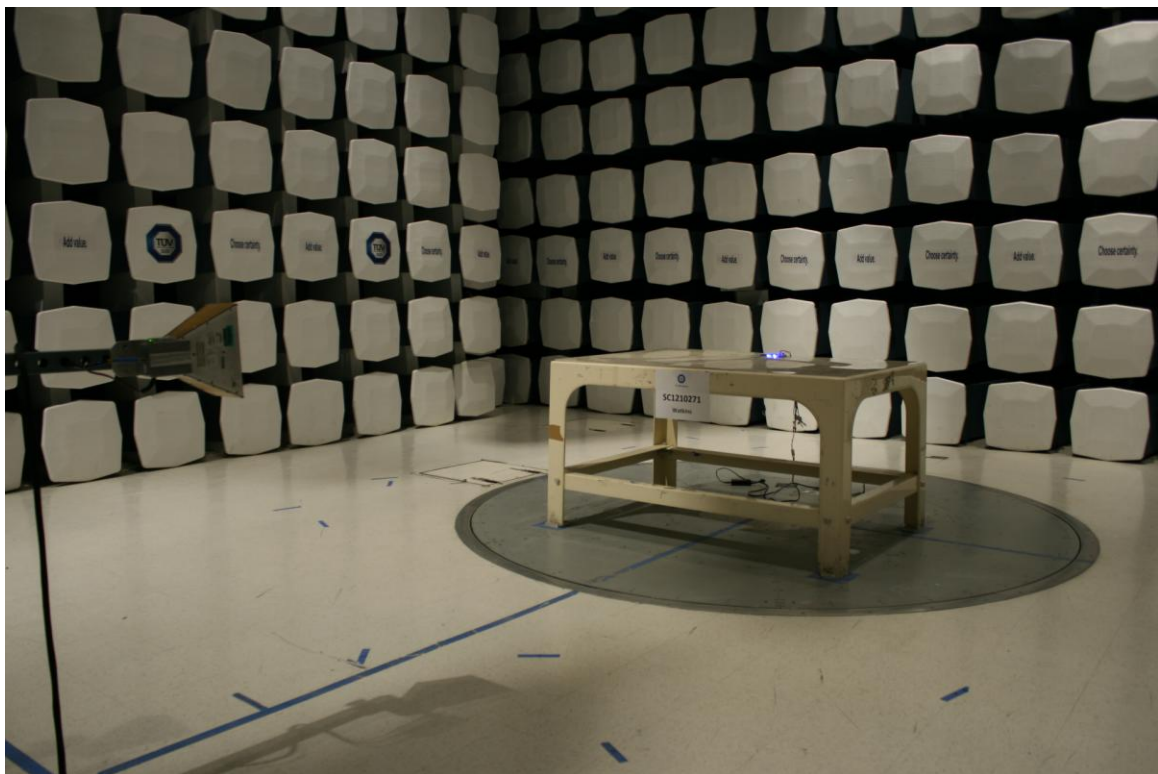
Radiated Emissions Test Setup (above 1GHz)
