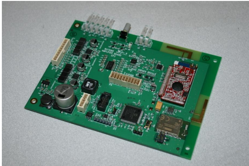
Equipment Under Test with PCB antenna
