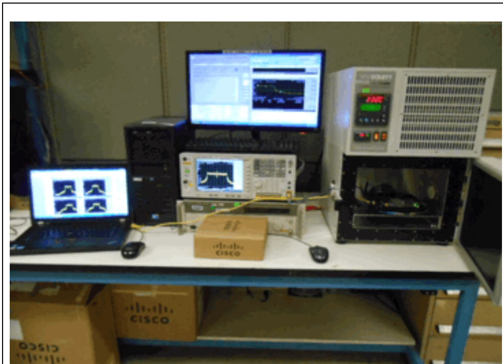
Title: Temperature / Frequency Stability Test Set Up
