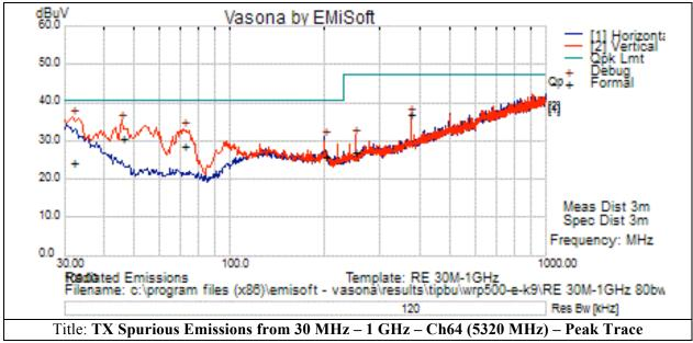
Note: The data displayed on the plots detailed in the graphical test results section were measured using a 'Peak Detector'. Please refer to the results table for the detectors used during formal measurements.
