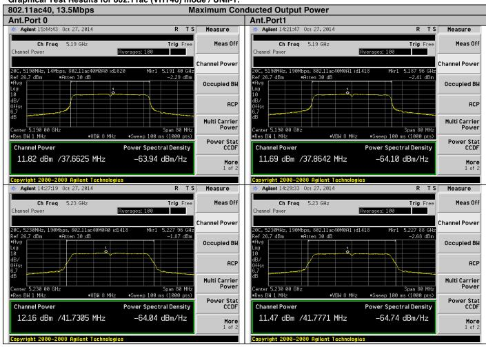
Graphical Test Results for 802.11ac (VHT80) mode / UNII-1
