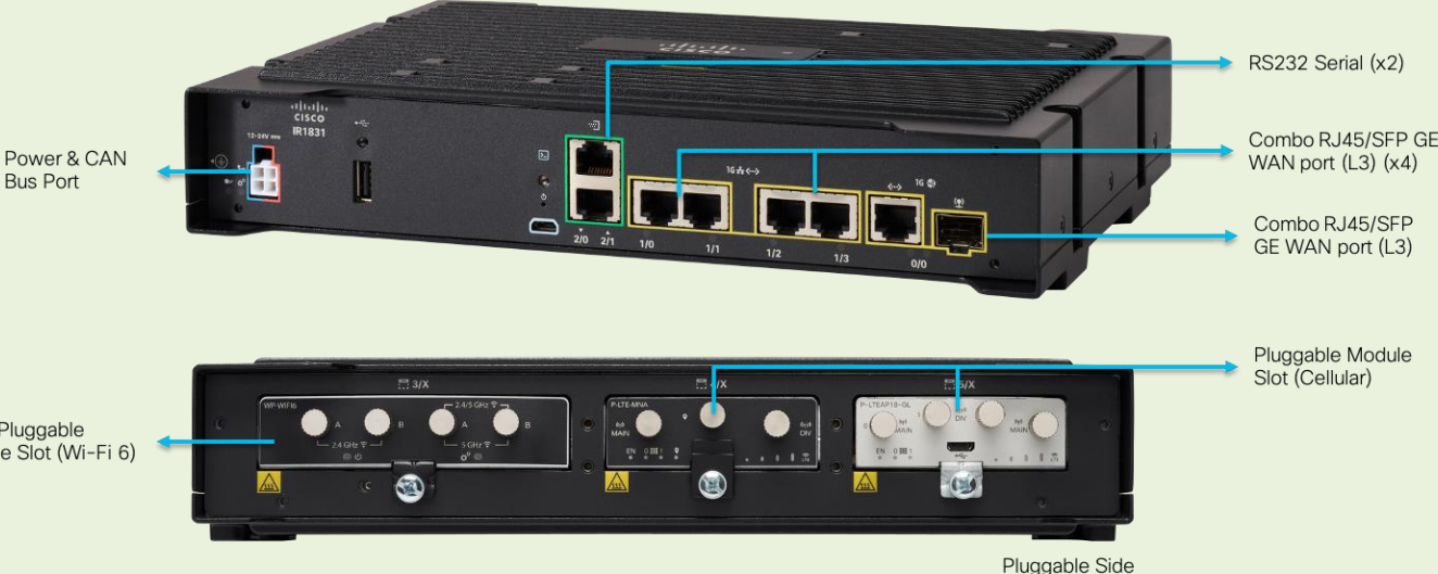
Figure 3. IR1831-K9 interface ports
