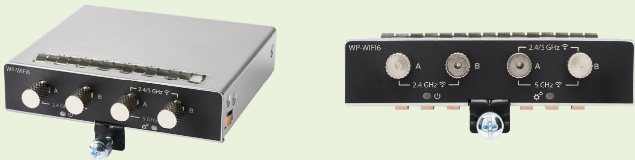
Figure 7. Wi-Fi 6 wide pluggable module
