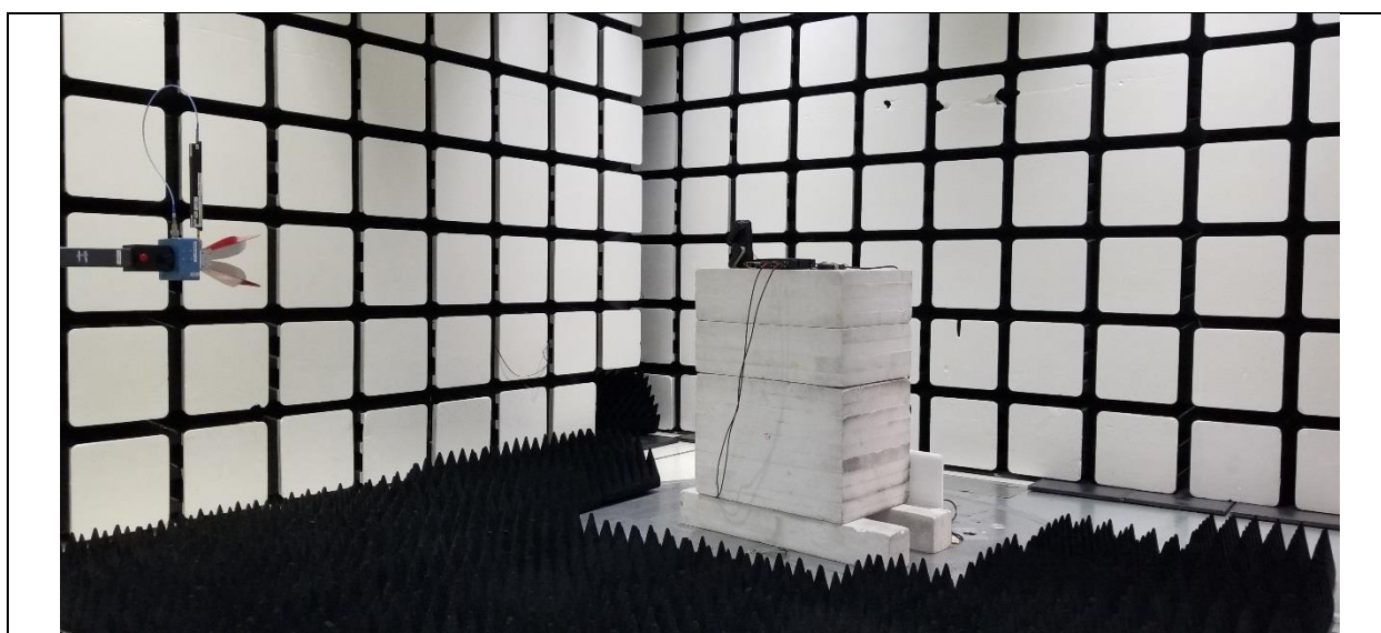
Title: Radiated Spurious Emissions Test Configuration 1G - 18GHz
