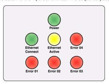
The ViperCell LED's are identified here. (The LED's on the ViperCell heatsink are not labelled).
