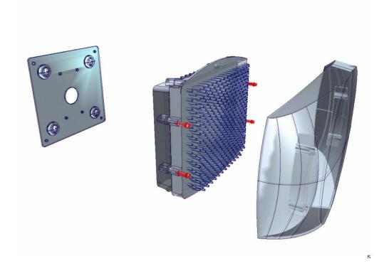
2 Gently press the Faceplate onto the ViperCell until the two clips snap into position on each side.
