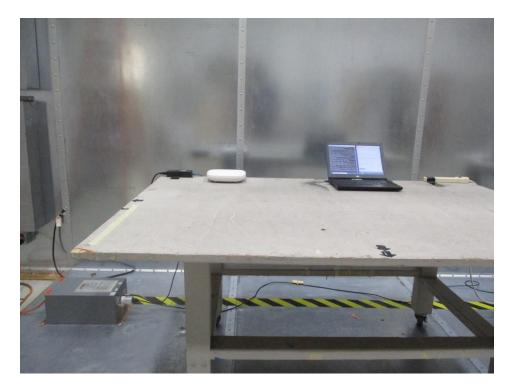
1.10 AC Line Conducted Emission Rear View
