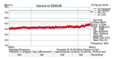
All emissions were below the average limit when measured using a peak detector. There were no emissions within 20dB of the peak limit.
