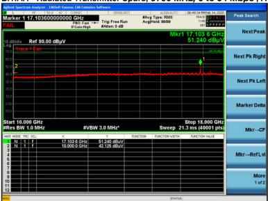
B.1.A.1 Radiated Transmitter Spurs, 5700 MHz, 6 to 54 Mbps, Average (10-18GHz)
