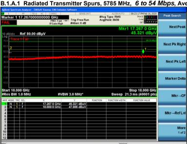
B.1.A.1 Radiated Transmitter Spurs, 5785 MHz, 6 to 54 Mbps, Average (10-18GHz)
