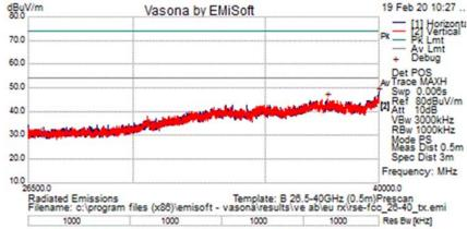
All emissions were below the average limit when measured using a peak detector. There were no emissions within 20dB of the peak limit.
