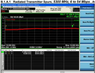
B.1.A.1 Radiated Transmitter Spurs, 5300 MHz, 6 to 54 Mbps, Average (10-18GHz)
