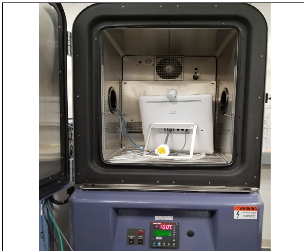
Title: RF Conducted Emissions Test Set Up
