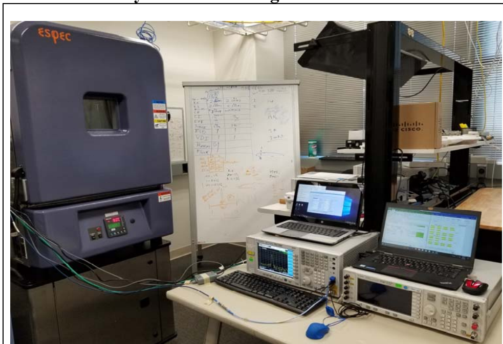
Title: RF Conducted Emissions Test Set Up
