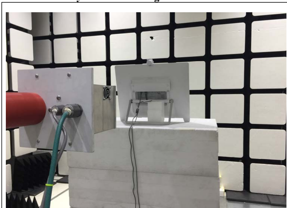
Title: Radiated Emissions 18 – 40 GHz Test Set Up
