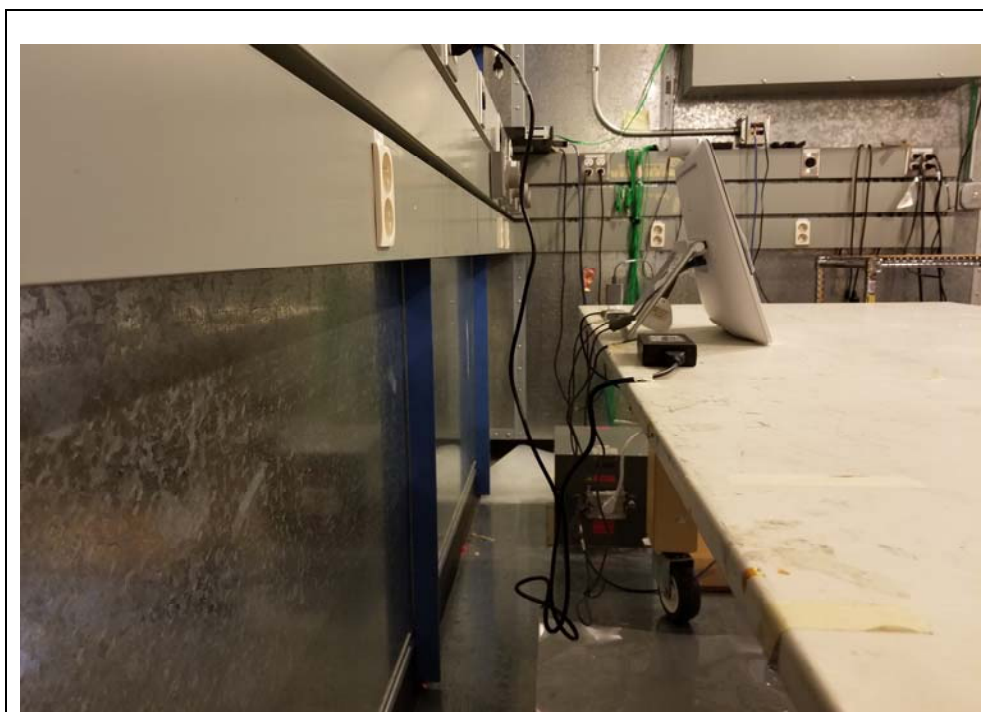
Title: AC Conducted Emissions Test Set Up
