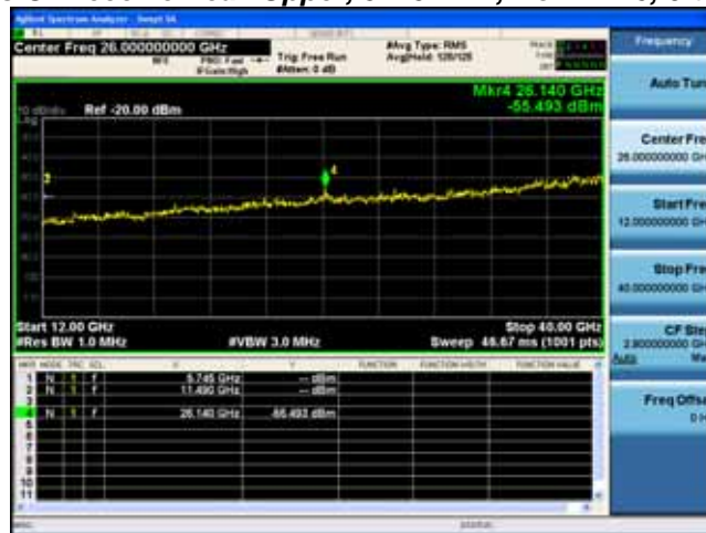
Spurious Of Receive Peak Upper, 5745 MHz, Non HT20, 6 to 54 Mbps
