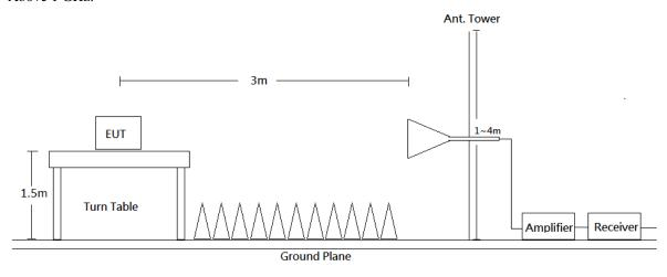
Radiated emission tests were performed in the 3 meters chamber test site, using the setup accordance with the ANSI C63.10-2013. The specification used was the FCC Part 15.209 and FCC 15.407 Limits.
