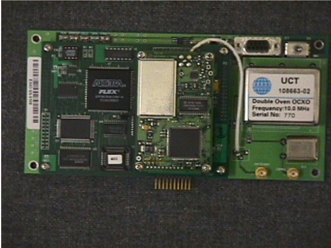
FIG 24. FRONTSIDE OF GPS RECEIVER (GPRS)
