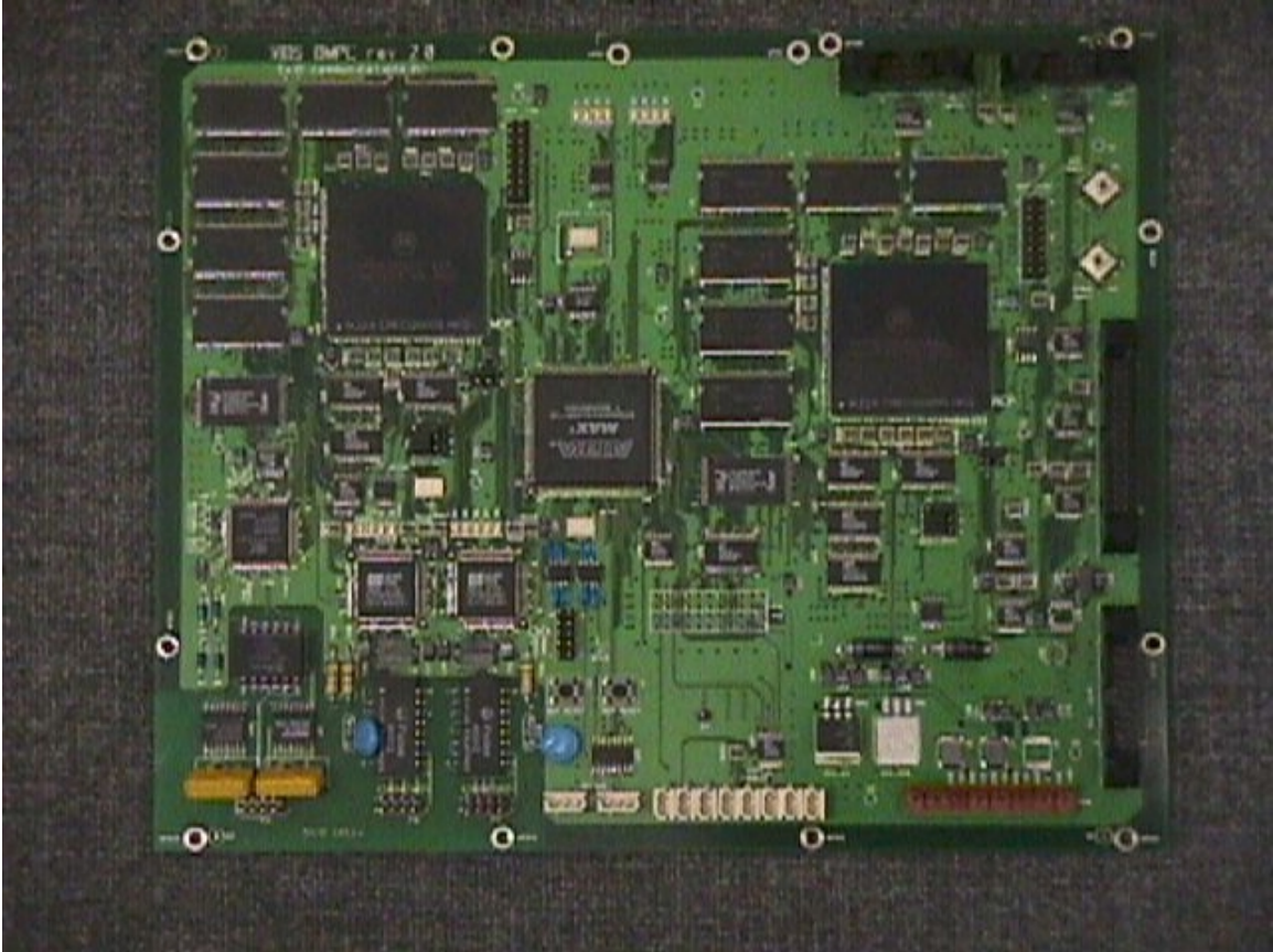
FIG 20. FRONT SIDE OF MAIN CONTROL BOARD (BMPC)
