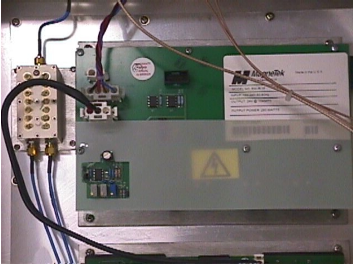
FIG 7. DUPLEXER (LEFT) FOR RX AND TX AND POWER MODULE
