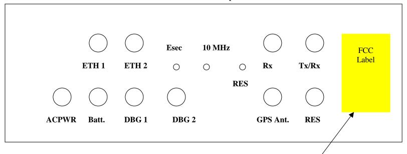
Label will be located on the bottom because MWIBS System will be located on the pole or wall bottom side will be the most visible side. Furthermore, installer have to see the bottom side because most of the port is on the bottom side
